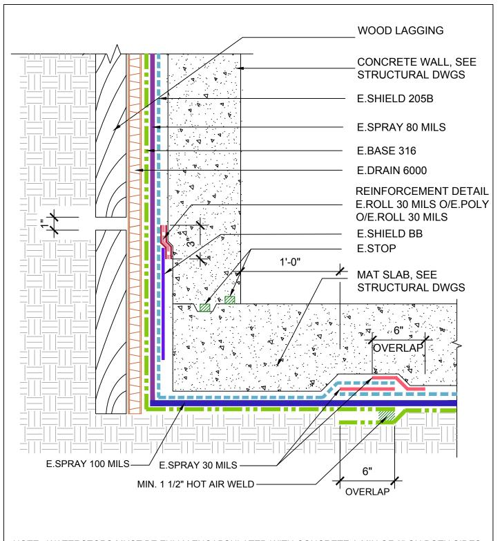
NOTE: WATERSTOPS MUST BE FULLY ENCAPSULATED WITH CONCRETE A MIN OF 3" ON BOTH SIDES
