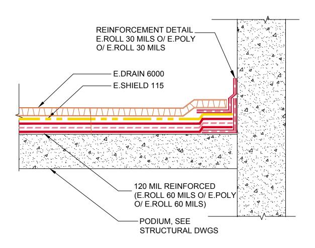
NOTE: APPLY REINFORCEMENT DETAIL PRIOR TO E.SPRAY AND AFTER INSTALLATION OF E.SHIELD 115
