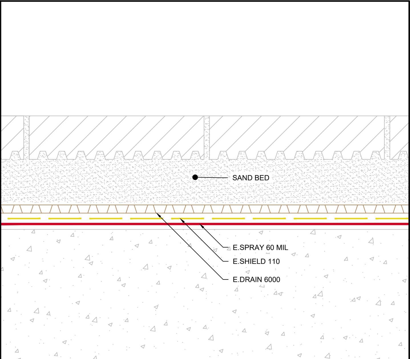
G:\My Drive\Epro Master Folder\Drafting\Details\Decks\E.Proformance\1.400.6 PAVER ON SAND BED DECK STANDARD ASSEMBLY.dwg [Detail] July 23, 2020 - 9:27am
